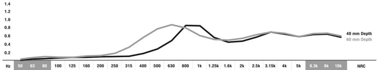
■ ABSORPTION COEFFICIENT: Values in accordance with the standards: EN 20654, ASTM C423 and EN 11654. ■ Values (<100Hz and > 5K) are Non Standard Values. \*PANEL DATA ONLY OF REF: QCK004 AND QCK006 MODELS.
